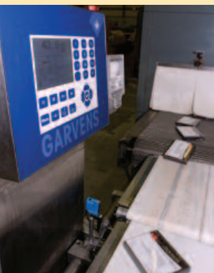
A specially-designed electronic scale monitors and verifies weights of individual samples as they roll through the addressing and shrink wrapping process at the new Bordentown production facility.
